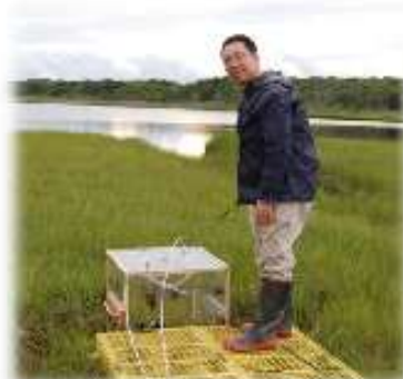
Gas chamber on marsh measuring greenhouse gas exchange between the salt marsh and the air.
