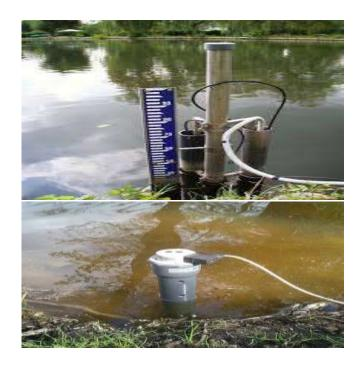
Water Level measuring device to calculate water depth
