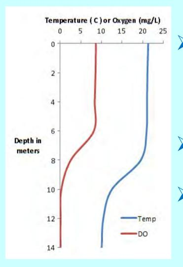
**Oxygenation is intended to:** Increase oxygen levels to avoid anoxia and accumulation of reduced compounds Provide deep water habitat with sufficient oxygen Maintain natural stratification; not mixing bottom and surface water
