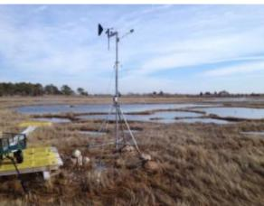
5/16/2013 At MET download, noted that the wind sensor was bent and stuck at 223 degrees.
